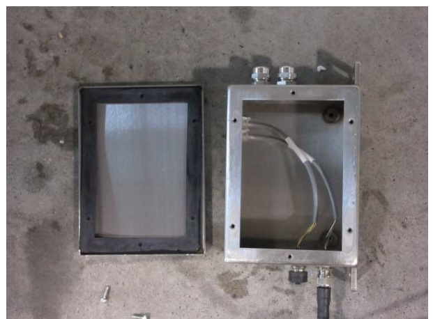
Fig 10: After IPX6 test, no water is visible in the enclosure of the sample
