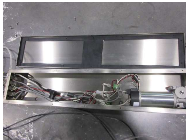
Fig 7: After IP6X test, no dust is visible in the enclosure of the sample
