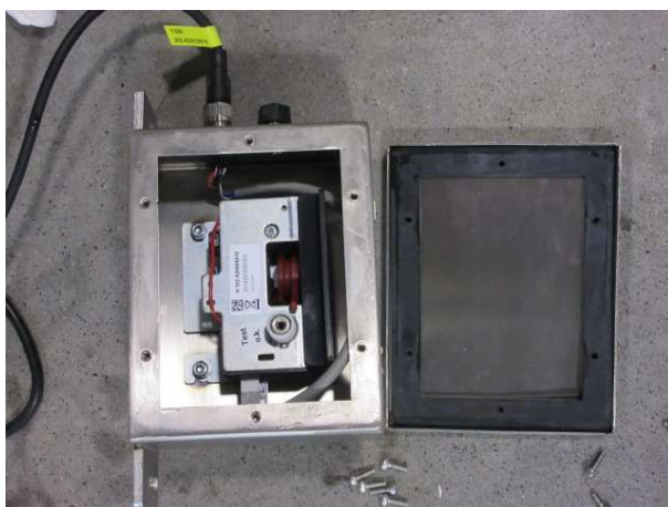
Fig 10: After IPX6 test, no water is visible in the enclosure of the sample
