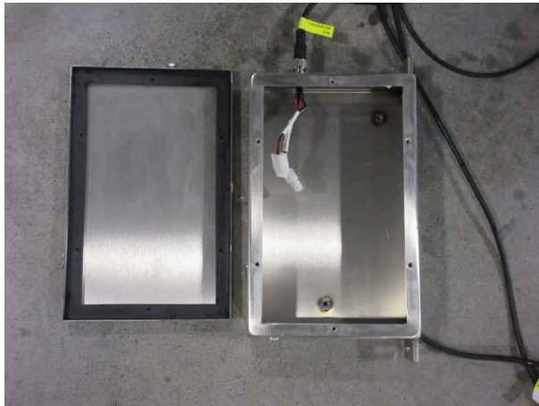
Fig 9: After IPX6 test, no water is visible in the enclosure of the sample
