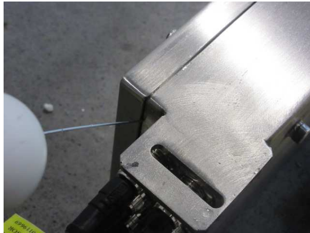
Fig 2: The object probe of 1mm \Phi does not penetrate the enclosure of the sample.
