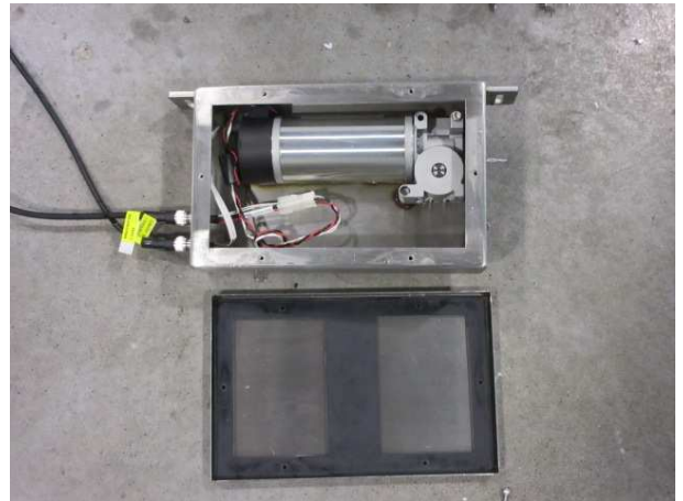
Fig 9: After IPX6 test, no water is visible in the enclosure of the sample
