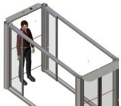
Move forward one step and remain between the door wings under the overhead door wing safety sensor for 5 seconds.
