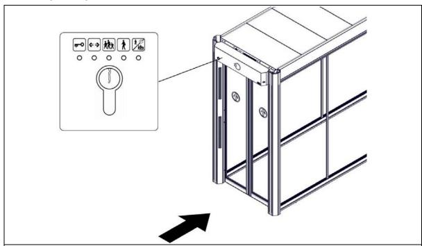
The control panel BDE-S (for the selecting the operating mode) is located in the on the cladding behind the cover of the entrance door.
