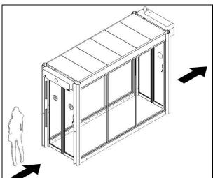
In the case of a main power failure, the UPS battery back up for the door will close the entry door and open the middle and exit doors regardless of the status of the safety sensors. Once the power is back, the FlipFlow will resume with the same operating mode selected before the power failure.
