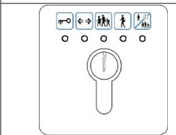
This control panel is used to switch between the various operating modes of the FlipFlow.
