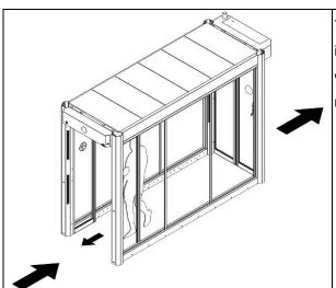
This alarm is triggered when the wrong direction is detected or if the entrance door does not close within a reasonable time (see below). A reset is required to deactivate this alarm.
