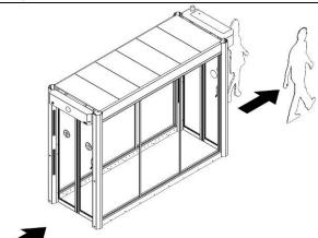
To increase the flow of persons and to minimize the eventual waiting time, the entrance door opens again, if the exit door is closed and the INTERLOCK is empty. After a short waiting time, the entrance door will close again. If another passenger enters the detection field of the tunnel, the FlipFlow will return to its normal INTERLOCK-Mode.
