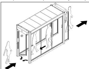
A person crosses the exit door threshold in the opposite direction, an alarm is triggered and the entrance door closes (TOF-Sensor).
