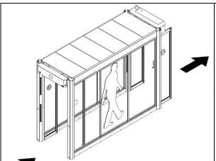
When this function is activated, the FlipFlow doors open regardless of the status of the safety sensors. This mode is activated in case of fire or emergency by a remote switch in the building management system. This switch is provided by the customer and will interrupt the connection between pin 3 and pin 4 on PM11 on the circuit board of each tunnel.
