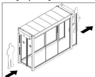
When this function is activated, the FlipFlow entry door will close regardless of the status of the safety sensors. This mode is activated by a remote switch in the building management system. This switch is provided by the customer and will interrupt the connection between pin 1 and pin 2 on PM11 on the circuit board of the first tunnel.
