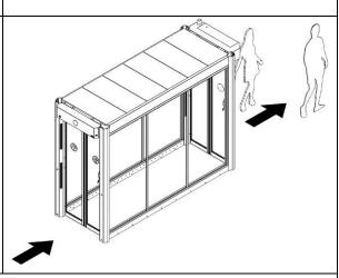
• The flow drops below the fixed threshold value the FlipFlow switches back to INTERLOCK mode and operates as described above.
